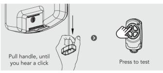
WARNING! Please test the manual release mechanism to ensure that the manual release is easy to operate. No more than 20kg of force should be required to disengage the door using the manual release cord. IF excessive force is required, contact your
