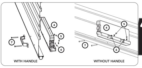
WARNING! To reduce the risk of damage to persons or property, be sure to cut off any excess thread of the screw that protrudes the weight bottle and file any burs.
